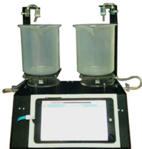
Figure 8. Photograph of the developed dual channel touch screen-based infusion pump analyzer.
