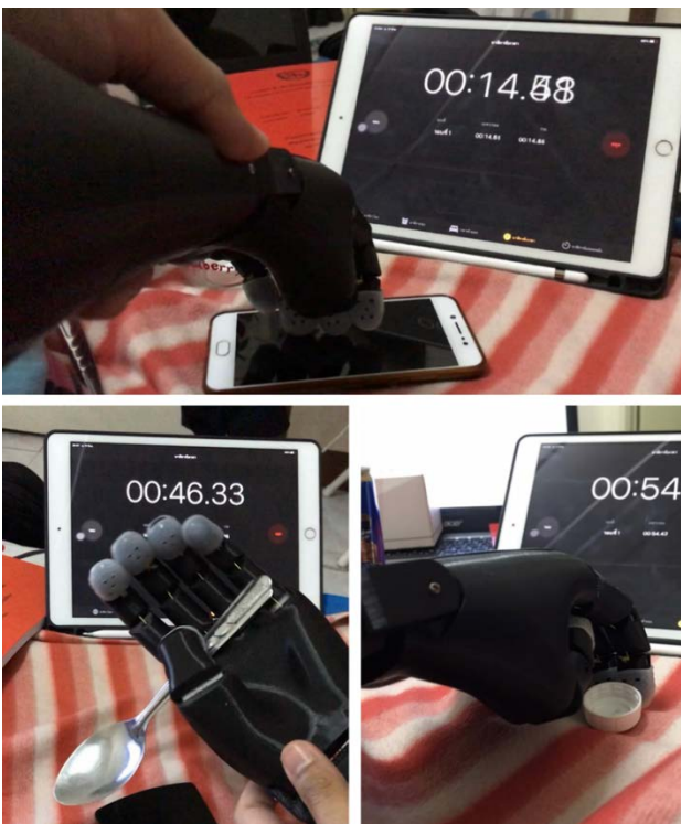
Figure 16. Fail of object holding experiment
