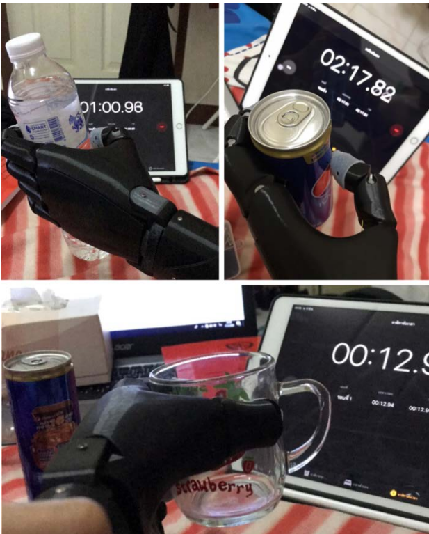
Figure 15. Success of object holding experiment
