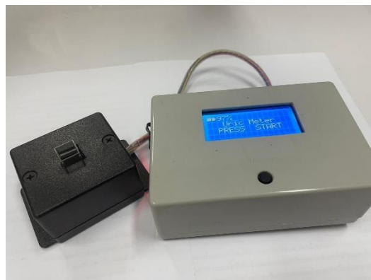
Figure 4. Prototype uric acid detector
