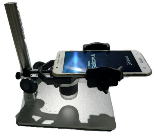
Figure 9. A microscope with a magnification of 400x used in research.
