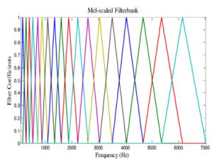
Figure 4. A Mel-scaled Filterbank [19]
