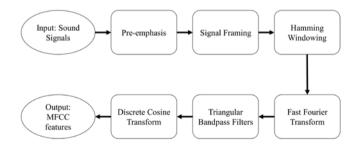
Figure 3. The Mel Frequency Cepstral Coefficients characteristic vectors extraction flow
