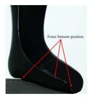
Figure 20. The position of force sensors in Para rubber slap.
