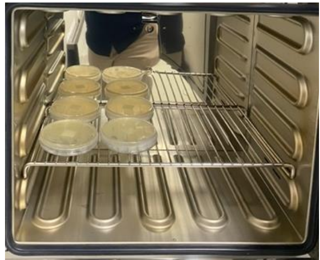
Figure 7 Cultivate and nurture microorganisms in an incubator at a temperature of 37 degrees Celsius for 7 days.
